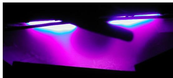
Fig. 11 Plasma shot showing unbalanced effect and linking of plasma for two magnetrons.
