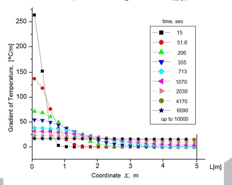
Gradient of Temperature at final instants of time (L = 5 m). D = 0.002 m<sup>2</sup>/sec,  $T_1 = 80^{\circ}$ C,  $T_2 = 0^{\circ}$ C,  $t_{MAX} = 10000$  sec. Final deviation of **grad T** from uniform value is less than 0.1%.
