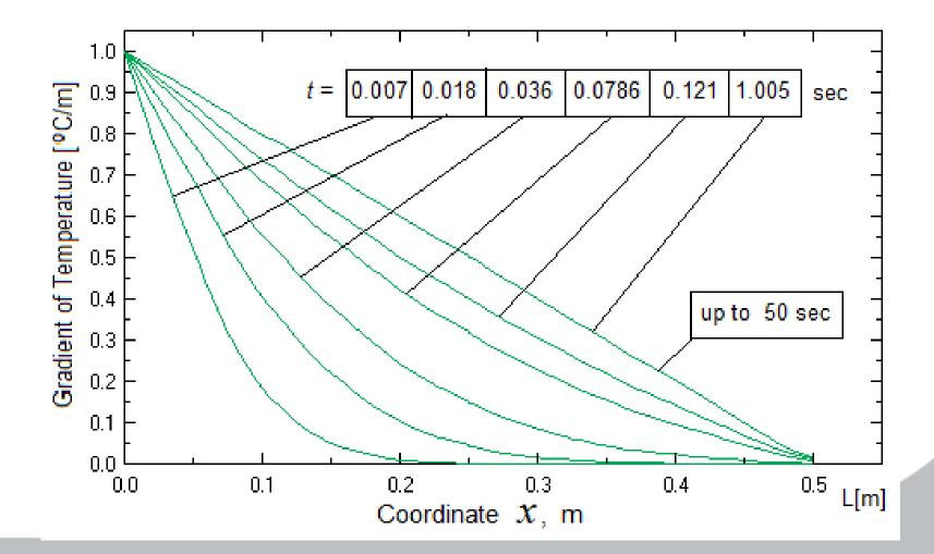
Temperature at the left edge of body at the constant value of heat flow.
