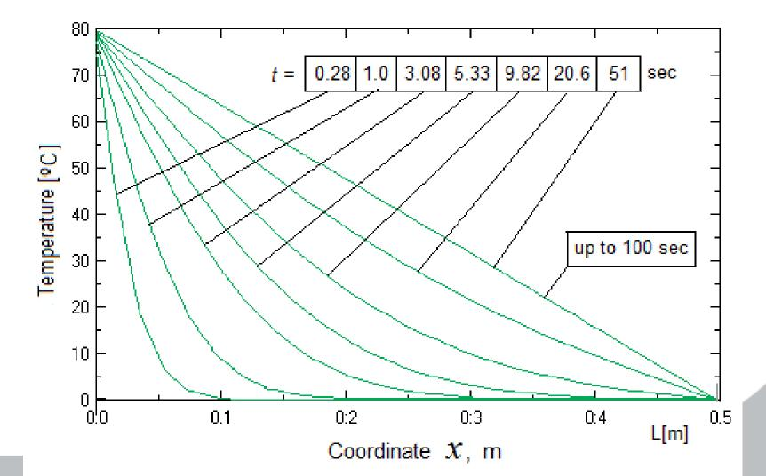
Gradient of Temperature for scaled model (L = 0.5 m). D = 0.002 m<sup>2</sup>/sec.  $T_1 = 80^{\circ}$ C,  $T_2 = 0^{\circ}$ C,  $t_{MAX} = 100$  sec. It is seen that with reduced length of sample to 0.5 m the heat flux automatically is increased in 10 times, what is general condition for the similarity of solution on the temperature.
