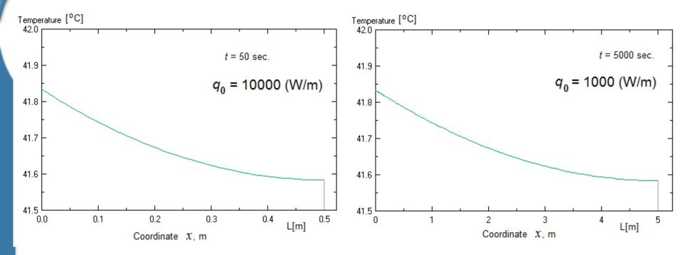
If we are able to reach a **similarity of process** on the base of criterion of similarity with a control of gradient of temperature equality **in the final instant of time for stationary state** of process, absolutely by the same way it is possible to reach the similarity for process at any another duration when the conditions of similarity for space and time parameters of models are fulfilled jointly with boundary conditions.
