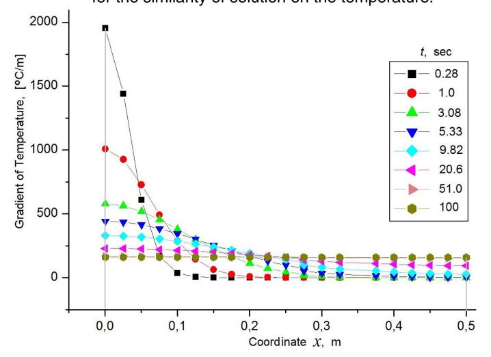
Gradient of Temperature at final instants of time (L = 0.5 m). D = 0.002 m2/sec,  $T1 = 80^{\circ}$ C,  $T2 = 0^{\circ}$ C, tMAX = 10000 sec. Final deviation of grad T from uniform value is less than 0.1%.
