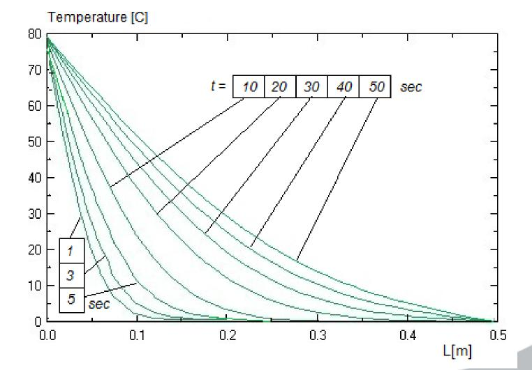
The absolutely similar distribution of temperature in the space and time is obtained at the next parameters: L = 5.0 m,  $t_{2MAX}/t_{1MAX} = 100$ ,  $X_2/X_1 = 10$ , D<sub>1</sub> = D<sub>2</sub> = 0.0005 m<sup>2</sup>/sec, saving the former boundary conditions.  $t_{2MAX} = 5000$  sec.
