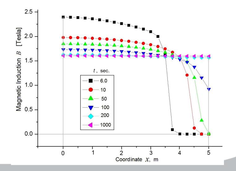
In the initial stage of process the steel has a zone of deep saturation with moving border of depth while in the rest part of sample steel is not saturated.
