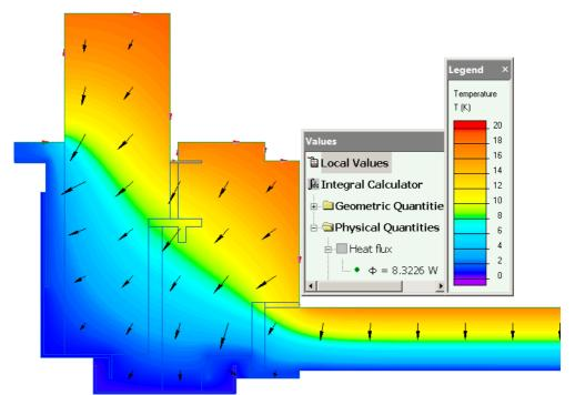
This automatically generated document consists of several sections, which specify the problem setup and finite element analysis simulation results. Navigation links in the top of each page lead to corresponding sections of this report.
