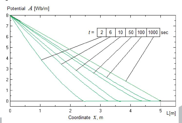
**Distribution** of magnetic induction along the Sample 1 (L = 5.0 m) has the specific zone of saturation with a moving border of depth. Process is going to the stationary state at  $t \rightarrow 1000$  sec.
