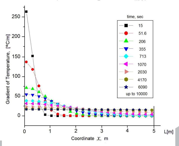
Gradient of Temperature at final instants of time (L = 5 m). D = 0.002 m<sup>2</sup>/sec,  $T_1$  = 80°C,  $T_2$  = 0°C,  $t_{MAX}$  = 10000 sec. Final deviation of **grad T** from uniform value is less than 0.1%.
