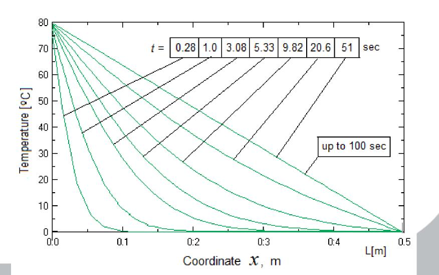
Gradient of Temperature for scaled model (L = 0.5 m). D = 0.002 m²/sec.  $T_1$  = 80°C,  $T_2$  = 0°C,  $t_{MAX}$  = 100 sec. It is seen that with reduced length of sample to 0.5 m the heat flux automatically is increased in 10 times, what is general condition for the similarity of solution on the temperature.
