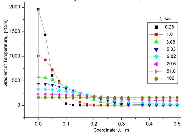
Gradient of Temperature at final instants of time (L = 0.5 m). D = 0.002 m2/sec,  $T1 = 80^{\circ}\text{C}$ ,  $T2 = 0^{\circ}\text{C}$ , tMAX = 10000 sec. Final deviation of **grad T** from uniform value is less than 0.1%.
