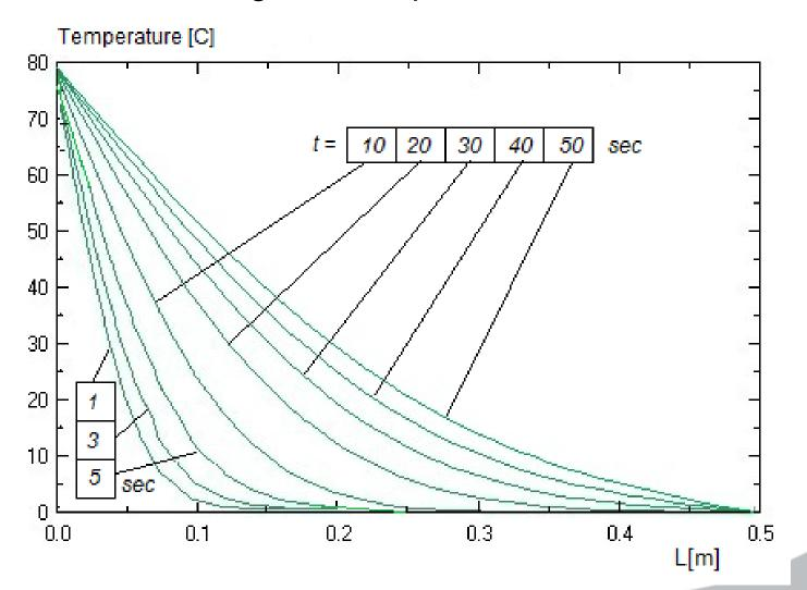
The absolutely similar distribution of temperature in the space and time is obtained at the next parameters: L = 5.0 m,  $t_{2MAX}/t_{1MAX}$  = 100,  $X_2/X_1$  = 10,  $D_1$  =  $D_2$  = 0.0005 m<sup>2</sup>/sec, saving the former boundary conditions.  $t_{2MAX}$  = 5000 sec.
