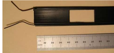
Twin-lead cable (actually a ladder line)
